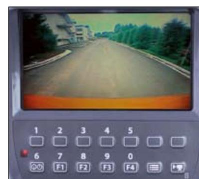
The widescreen color LCD, teamed up with the rear view camera on the counterweight, gives the operator unobstructed rearward viewing. The rear view camera automatically works when traveling, and can also be manually turned on with a select switch on the monitor.
