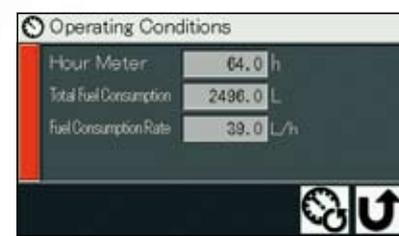
Fuel consumption per operating hour is computed, and the result is displayed on the LCD monitor. This information suggests refuelling timing, and guides energy-saving operation and efficient job management.
