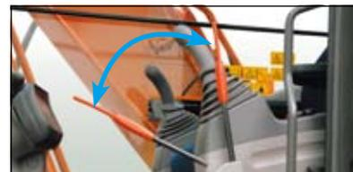
Other features include a retractable seat belt, evacuation hammer and emergency engine shut-off switch. A shut-off lever for pilot control helps to prevent unintentional movements.
