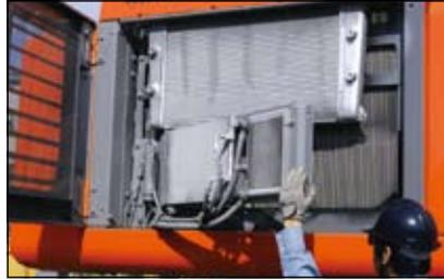
The radiator and oil cooler are laid out in a parallel arrangement, instead of the conventional in-line arrangement. This parallel arrangement is significantly easier to clean around the engine. The air conditioner condenser can be opened for easy cleaning of the condenser and the radiator located behind.
