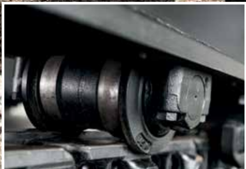
Strengthened bushing material improves wear resistance.
